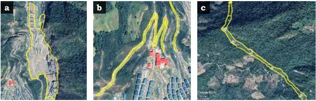
Figure 1. Manual delineation of (a) infrastructure, (b) road, (c) transmission line
