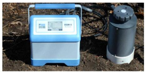
Figure 11: Equipment to measure the soil respiration or carbon efflux
