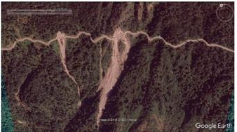
The debris from road construction and maintenance are mostly dumped below the road (Figure 12) without proper guidance and care. The debris and boulders along the steep terrain often fall into the streams and rivers and increase the sediment load contributing to heavy bed loads along the downstream. Sometimes, during the peak rainy season, the
