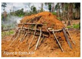
system of this type of kiln is difficult to control, the carbonization process is incomplete, resulting in production of low quality charcoal. However, in some parts of the world, the earth kilns are improvised by fitting a chimney to allow better control of air flow and reduce heat loss during carbonization, producing higher quality charcoal. The earth kiln must be completely rebuilt after each cycle and the production cycle lasts around 24 hours which is too long.
