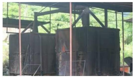
Figure 6: Metal Kiln for Charcoal Production fuelled by firewood
