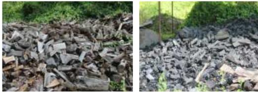
*Figure 4: Firewood chipped into appropriate Figure 5: Charcoal (finished produce) sizes for use as raw material*
