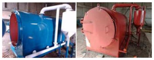
Figure 11: Semi-automated Charcoal Production Kiln
