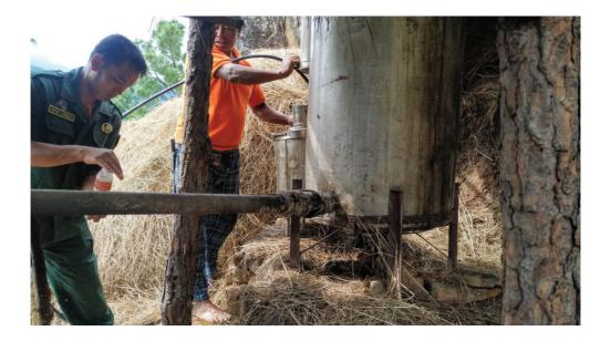
Pictured above, Demonstration of extracting lemon grass oil using a distillation drum.
