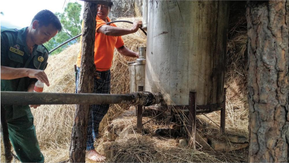
*Pictured above, Demonstration of extracting lemon grass oil using a distillation drum.*
