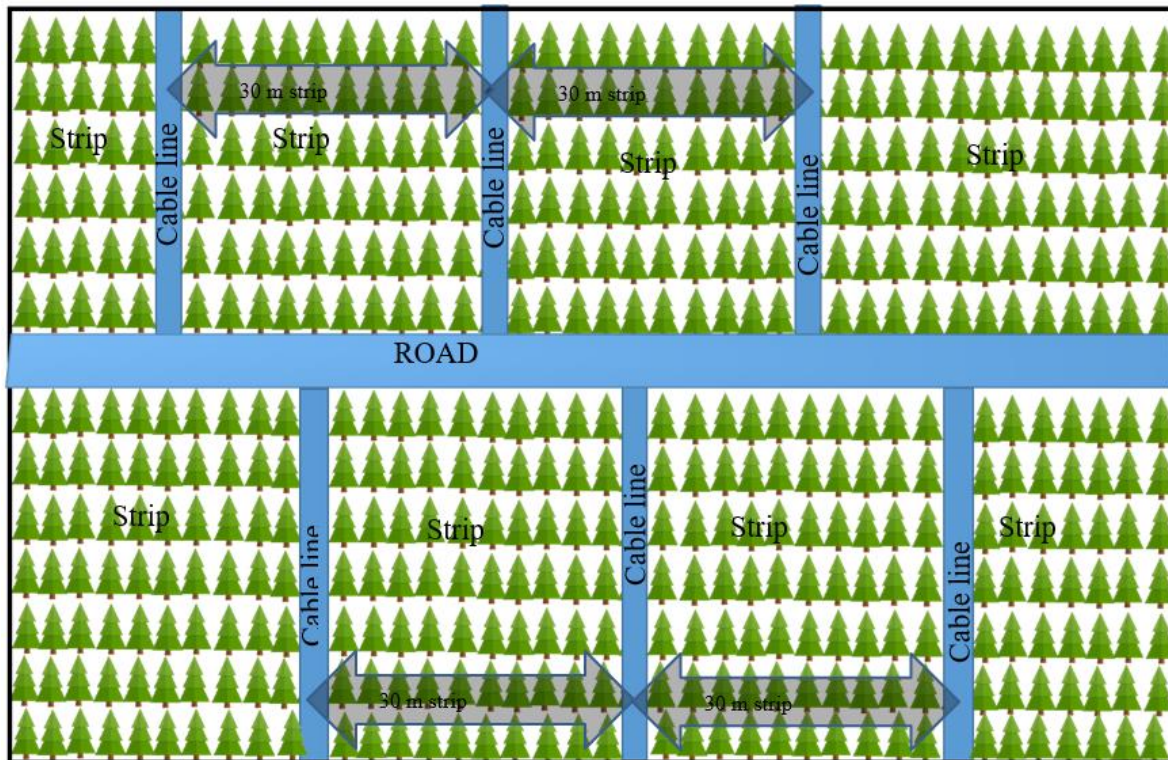
Figure 8.2: Layout of the cable lines
