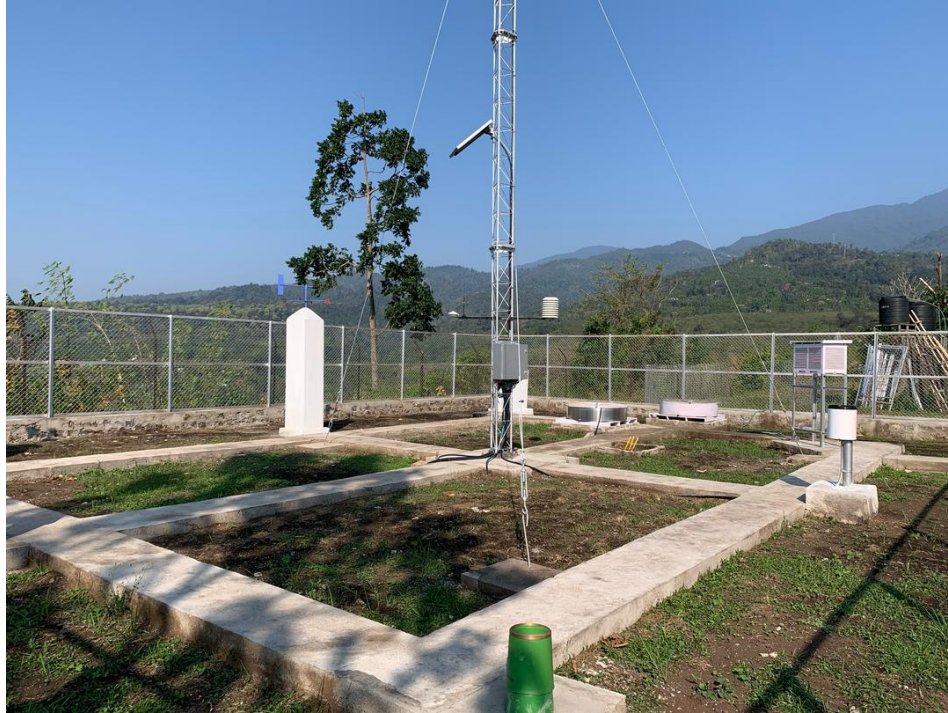
Figure 3: Samtse Automatic Weather Stations with Manual stations with completed civil work
