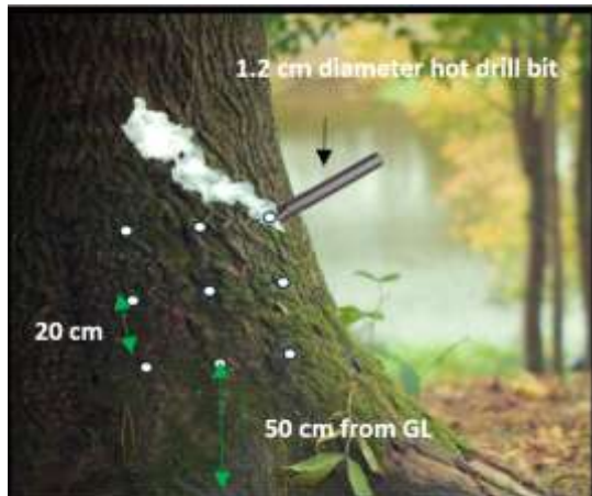
Figure 12: Burning chisel drilling technique
