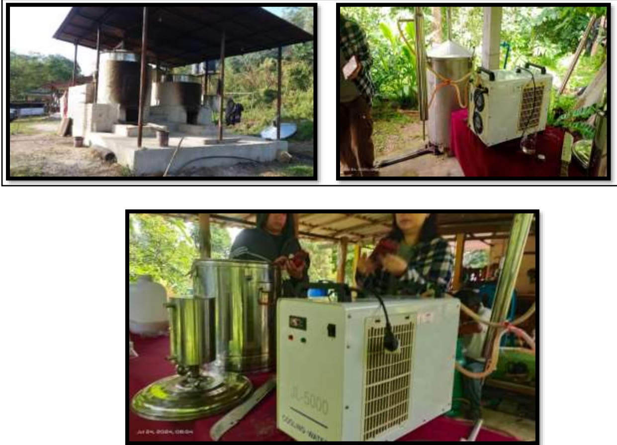
Figure 25: Distillation units 1. Firewood heating, 2. LPG distillation unit and 3. Electrical distillation unit.
