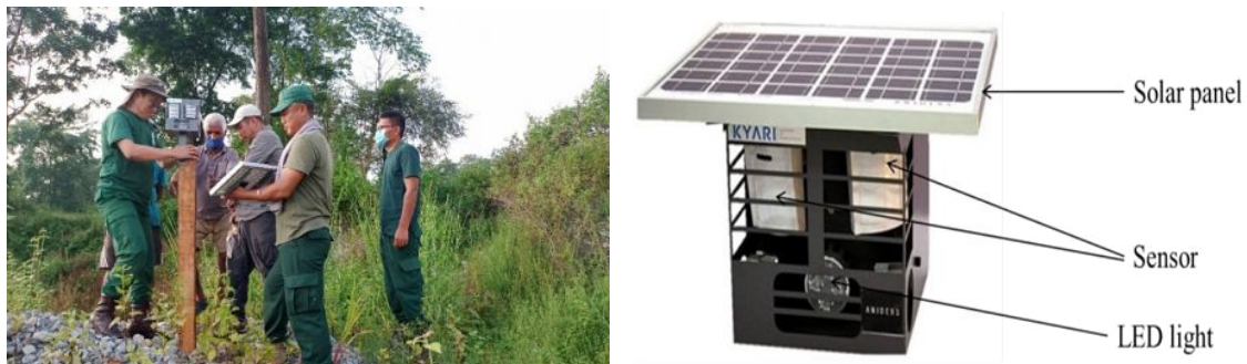
Figure 40: Animal intrusion detection and repellent system (ANIDERS).
